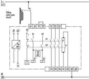
The single channel protective gate application complies with the requirements of the Stop-Category 0 acc. to EN 60204-1 and the Safety Category 2 acc. to EN 954-1. However the circuit of the protective gate is not redundant. Ground faults in the protective gate contact are immediately detected.
