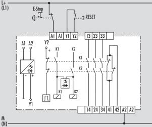
The single channel E-Stop circuit complies with the requirements of the Stop-Category 0 acc. to EN 60204-1 and the Safety Category 2 acc. to EN 954-1. However the circuit of the E-Stop momentary contact is not redundant. Ground faults in the E-Stop circuit are immediately detected.
