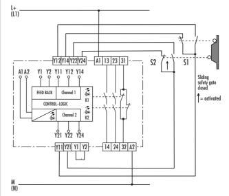
Channel 1 (Y11) and channel 2 (Y21) monitor the position of the sliding protective gate. The SNZ 4052 K is activated with an automatic START. If the sliding protective gate opens, the two-hand relay switches back to their off position (enable current paths 13/14, 23/24 are opened). If the protective gate is closed again, the automatic START activates the two-hand relay again.
