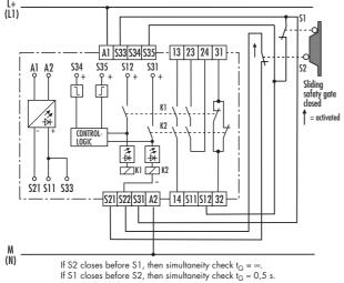
Channel 1 (S12) and channel 2 (S22) monitor the position of the sliding protective gate. The automatic START through terminal S35 activates the SNO 4062 K/SNO 4062 KM. If the sliding protective gate opens, K1 and K2 switch back to their off position (enable current paths 13/14, 23/24 are opened). If the protective gate is closed again, the automatic START at S35 activates the device again.
