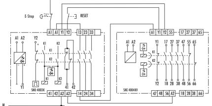
Single - Channel Emergency - Stop Application with Contact Expansion. Basic Unit SNO 4003 K with Expansion SNE 4004 K.
